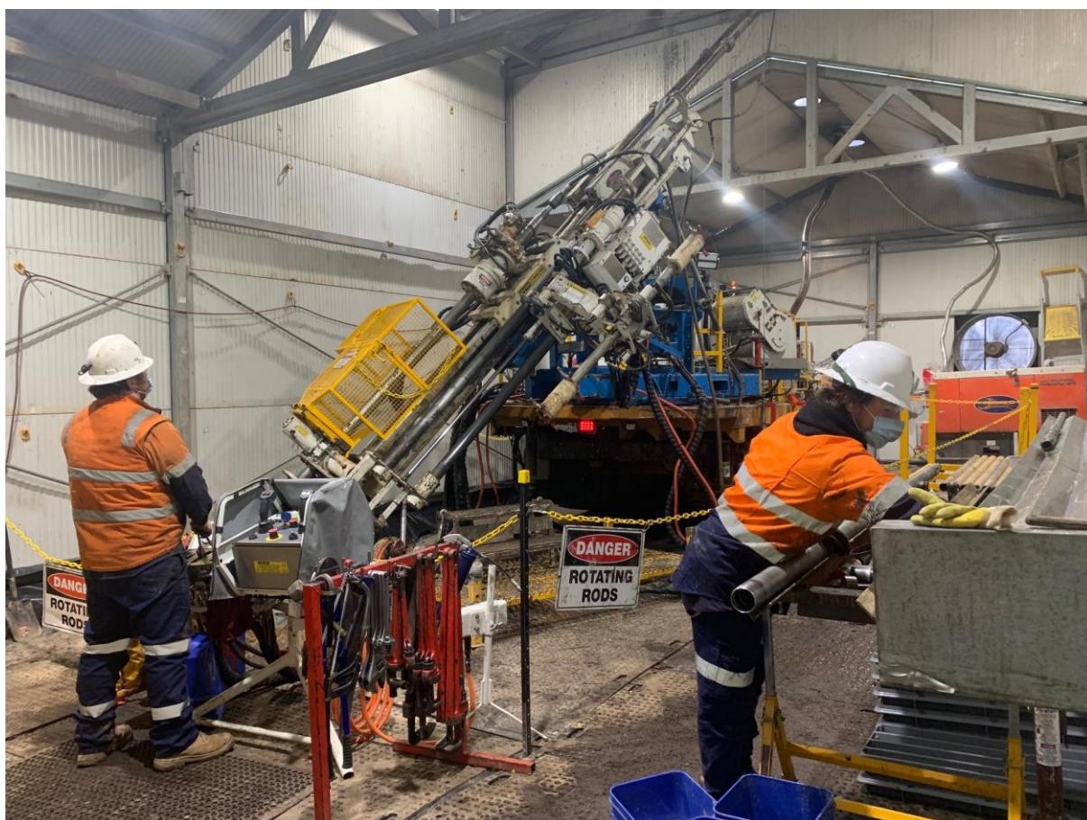
Figure 2: Current diamond drilling operations at Resolution Lode on the east flank of the Irvine basalt dome.
