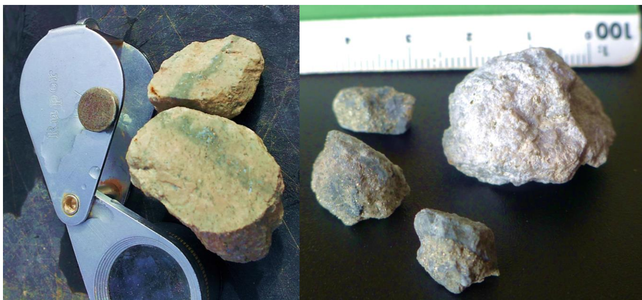
Figure 3: Examples of bleached, altered drill chips intersected in drilling showing fine-grained disseminated sulphides.
