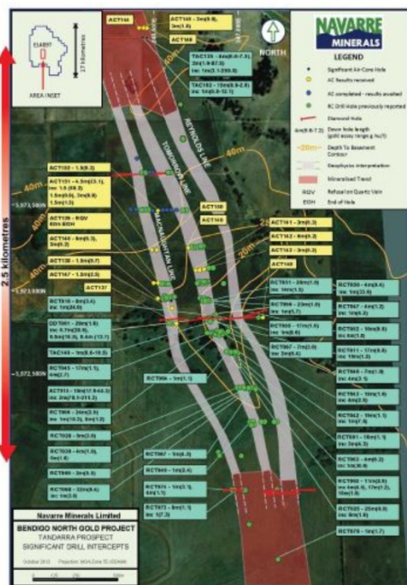
Satellite image of part of the Tandarra prospect showing near surface gold mineralisation trend, its projection to the north and south and location of air-core drill holes. Source: Company announcement
