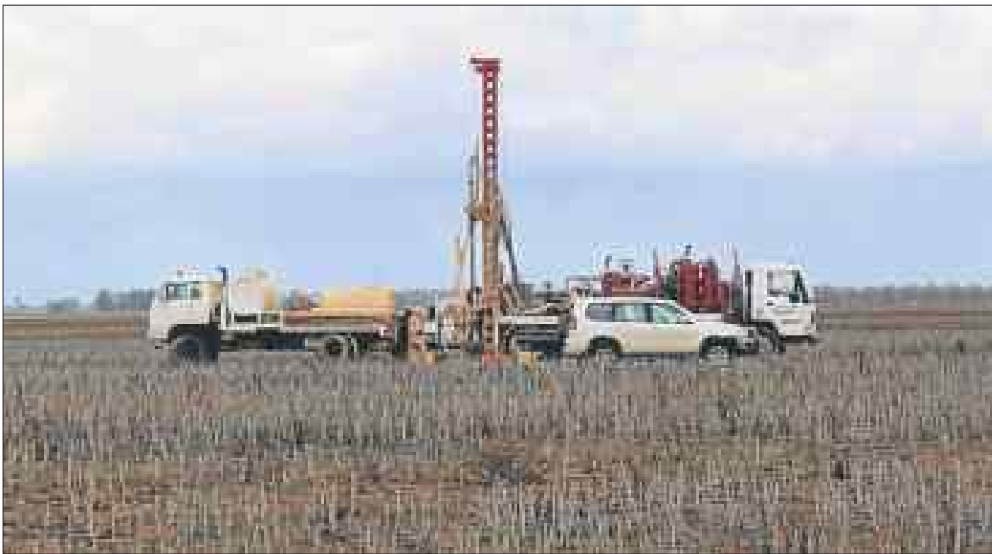
Air-core drilling being undertaken at the Tandarra Gold prospect by Navarre Minerals.
